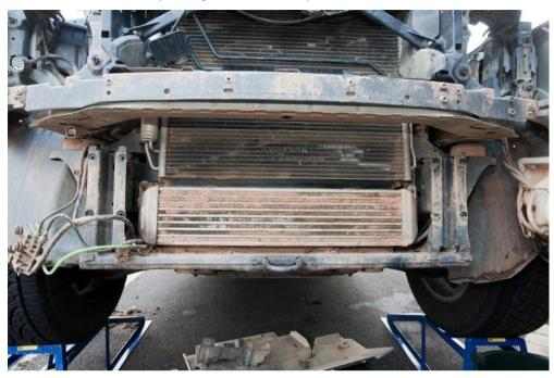
You can now wiggle the air duct out to give you access to the intercooler.
