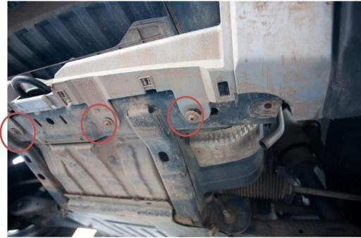
On each side of the bumper, there is a screw that should also be removed.
