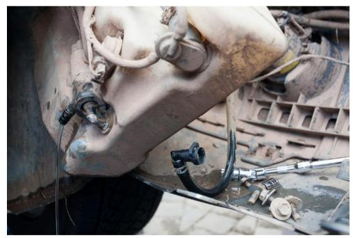
Next, remove the two cover plates giving access to the intercooler hose connections.
