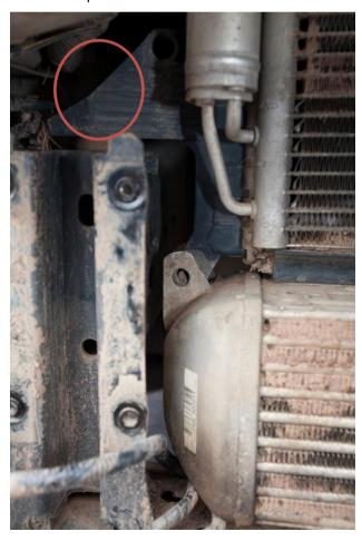
Using a crow bar, lift the radiator enough to release the intercooler from its bracket. The intercooler will slide across to give a little more room to help its removal. The picture below shows where the bar is located to lift the radiator. (After the new one was fitted)
