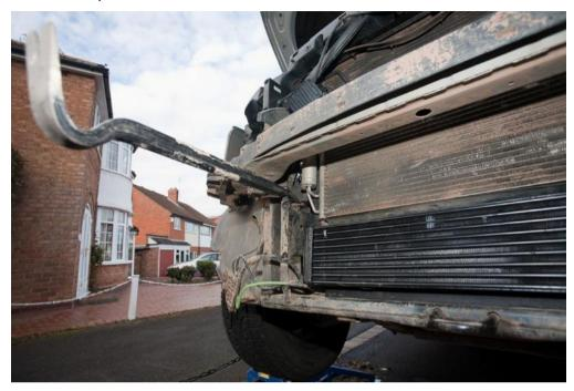
Once the old intercooler is removed, clean around the area to remove the mud and dust.
