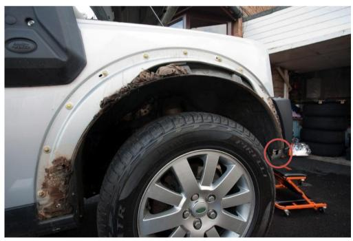
At the front leading edge of the arch, there is a plastic Tee which slots into the bumper – care needs to be taken not to cause damage. The slot is shown ringed in red.
