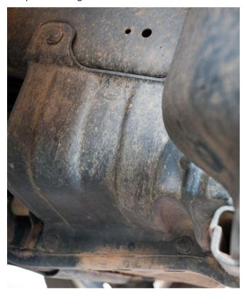
Now the right hand cover is removed, it is possible to access the second screw holding the air duct into the car.
