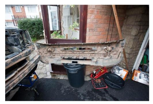
The next stage is to remove the metal bumper bar. Before doing that, the washer bottle needs to be unbolted from the one end and the control box from the other.
