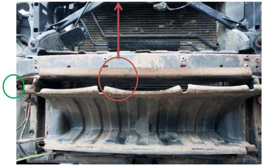
The sensor needs to be disconnected at the point shown in the Green circle above.
