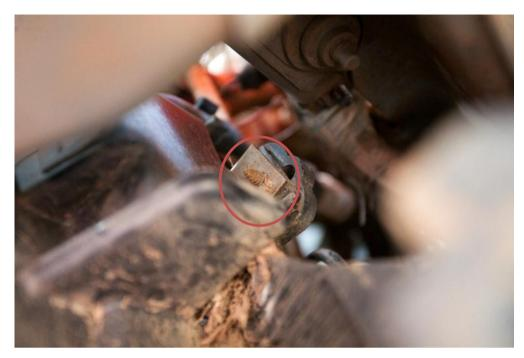
To remove the washer bottle, remove the two remaining fixings. A 10mm socket and universal joint and extension bar will be required.
