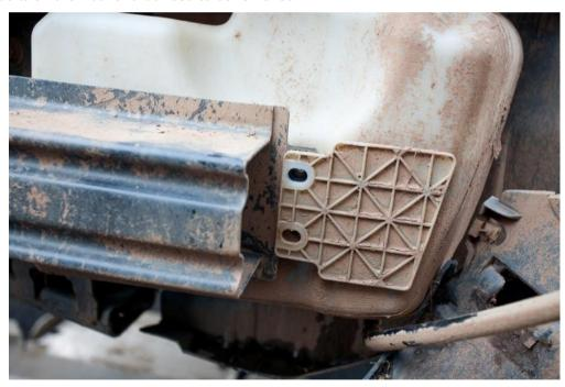
The suspension control box is just lifted up and off.
