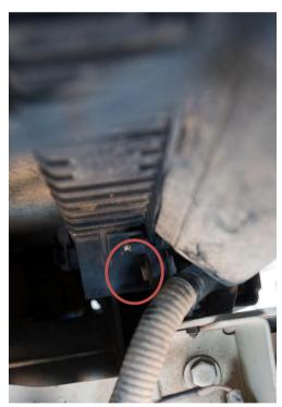
The screw on the other side is not so easily accessed. The picture below, is taken looking up from the front of the car, once the washer bottle has been removed.
