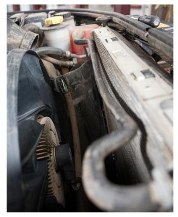
Once the side cover is unclipped, return to the underside of the car and unclip the two clips that hold the radiator cowl onto the intercooler.
