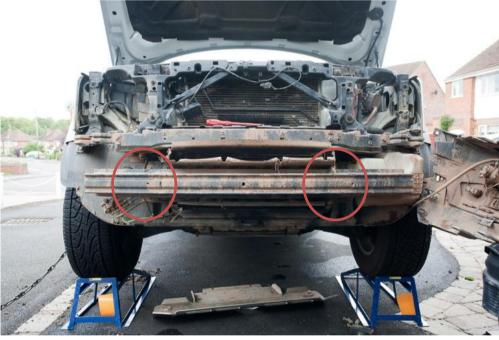
There are 4 13mm bolts each side, which hold on the bumper bar. You can undo all the bolts without fear that it will fall off, because there is a clip that holds it onto the bracket. One of the bolts also holds the washer bottle.
