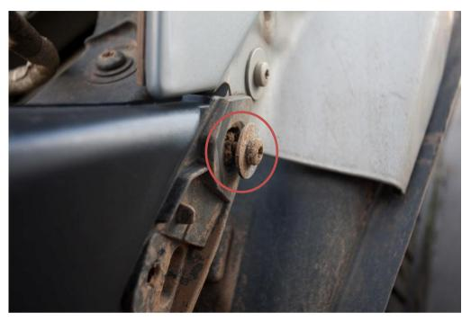
Before removing the bumper, if you have fog lamps and/or PDC, disconnect the plugs, located on the left hand side as you face the car. I used a screwdriver, as seen below, to release the clip.
