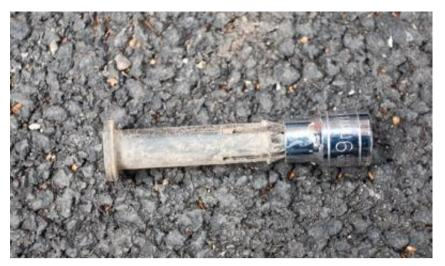
The picture above shows the principle using the socket on the end of the sleeve to compress the end. From under the car, remove the two clips that hold on the hoses to the intercooler.
