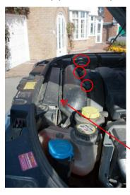
The top cowl can then be removed once the top vent hose is also unclipped. It needs to be pulled up – but be very careful that the jubilee clips around the various pipes don't attack you and rip your finger open. ©
