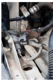
At the back of the expansion tank, is the hose to the system and at the top the return from the far side of the radiator. At the very bottom of the tank is the level indicating switch – a metal clip holds it in. The plug is shown in the last picture above.
