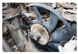
If you don't take the fan off, then you need to release the fan from the viscous unit – it's four 10mm screws, which are accessed from the back. With the fan like this, there is just enough room to get the access needed to remove the pipes.
