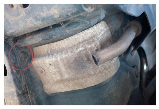
Again, these are held on with the plastic self locking clips. One is circled above. The picture above is the right hand one, with the metal heat shield for protection against the FBH exhaust.
