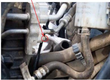
Another screw about 2/3<sup>rds</sup> down the right hand side also needs removing. Both of these screws are by the main holding bolts for the radiator.
