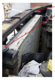
They are removed by releasing the clip with a small screwdriver at the top of the radiator where the pins go in – the pins have an arrow showing the location of the release.
