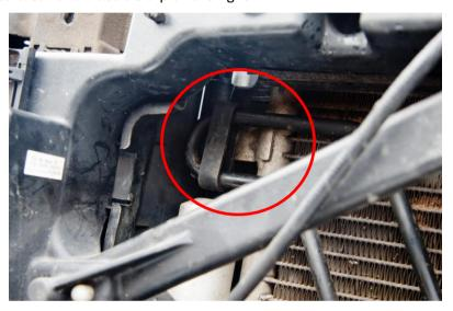
There are a couple of screws that hold the air conditioning condenser onto the radiator – top and 2/3<sup>rds</sup> down on the left and middle right, together with a screw where the two pipes come from the AC system also on the right.
